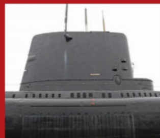
Left: The conning tower was replaced after the 1958 refit as the Alliance's role changed to a sub-hunter
